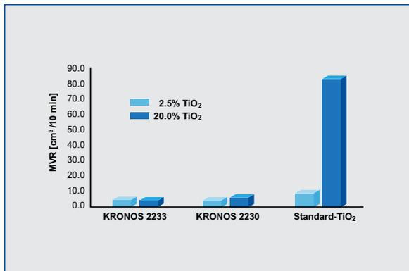
Fig.2 MVR values (300°C/1.2kg) as a function of TiO<sub>2</sub> content
